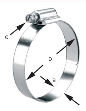
C (screw type) = C8 hexagon slotted screw sw 8 Diameter D = 83-105Width B = 16
